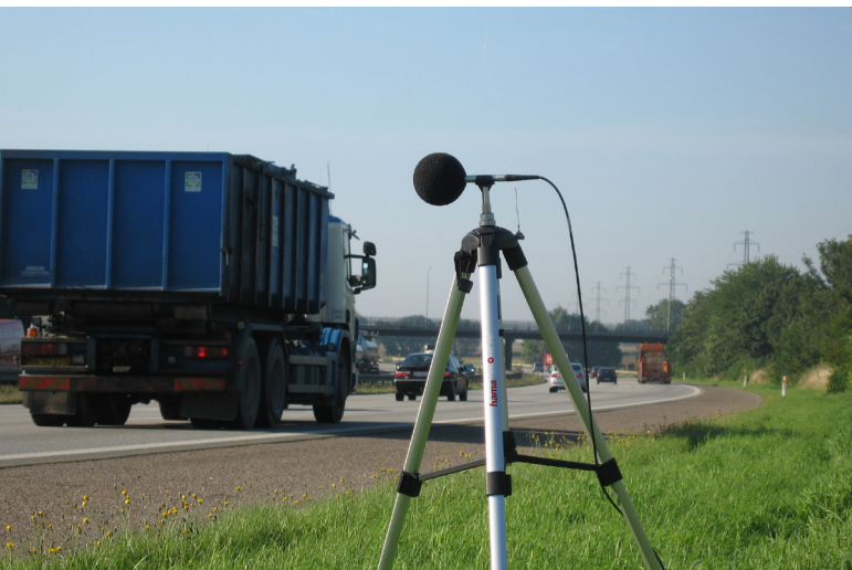
Figure 4: A microphone along the road for pass-by measurements. The microphone is placed close to the road and measures noise from passing passenger vehicles and lorries.
