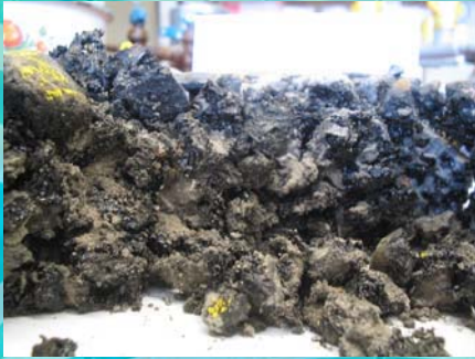
Example of profile of a drilled SLPA core
