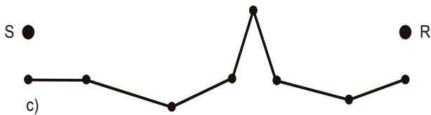
FIGURE 2. Vertical terrain cross-section simplified to straight-line segments (Plovsing, 2006a)
