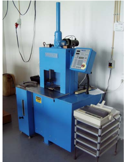
Figure 5b. Troloxer Gyrotory Compactor at Danish road Institute.
