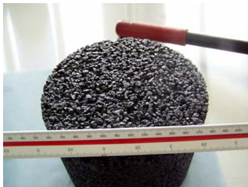
Figure 5c. Gyrotory compacted specimen of SMA -LN 6.
