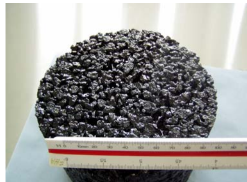
Figure 5d. Gyrotory compacted specimen of SMA -LN 8.
