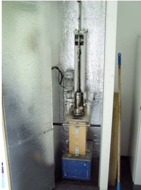
Figure 5a. Marshall compaction equipment in its noise reducing cupboard at Danish Road Institute.
