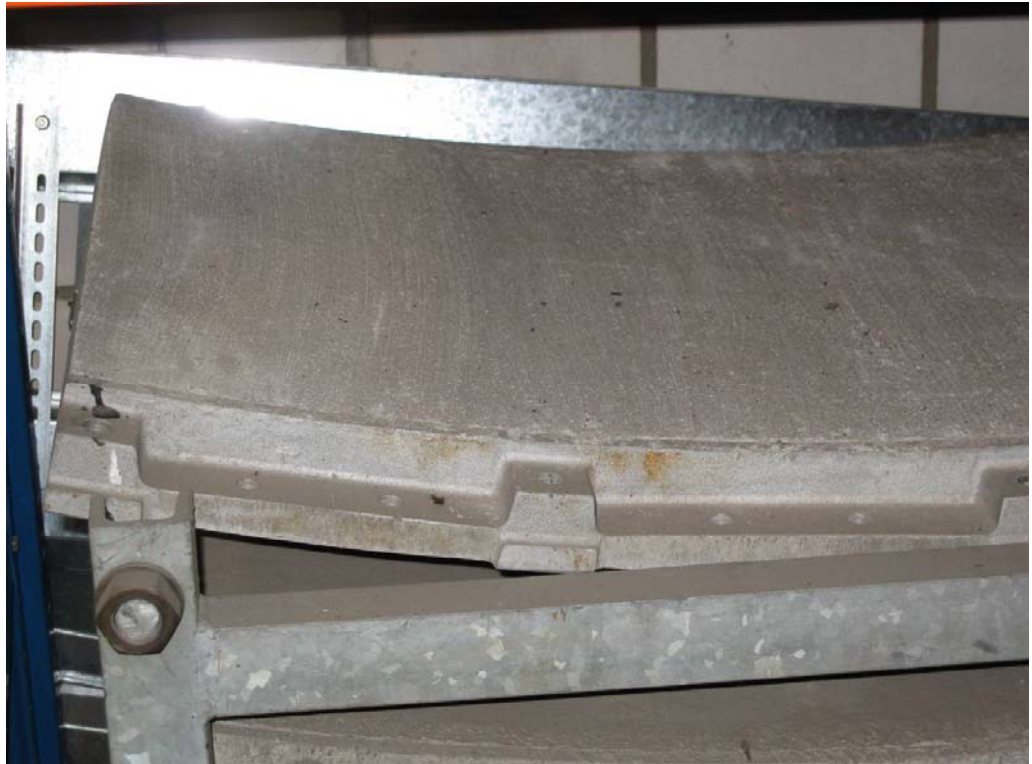
Figure 2. Mould to be filled with pavements to be tested.
