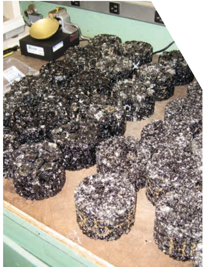
Figure 1.2: Cylindrical Marshall specimens of the 12 mixes produced in the UCPRC laboratory in California.
