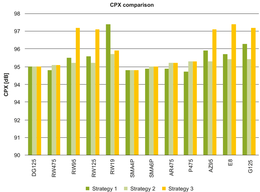
Figure 7.1: Comparison of the CPX results using the three different AOT prediction strategies.
