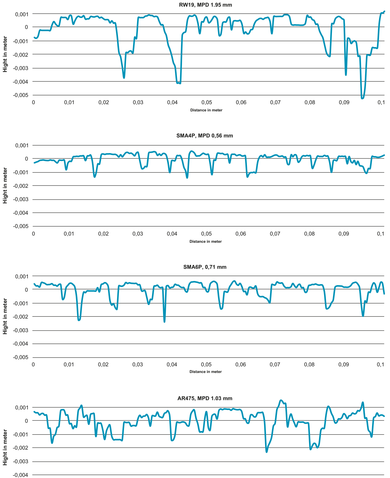
Figure 5.2: Randomly selected 10-cm long sections of these texture profiles for each of the 12 pavements.
