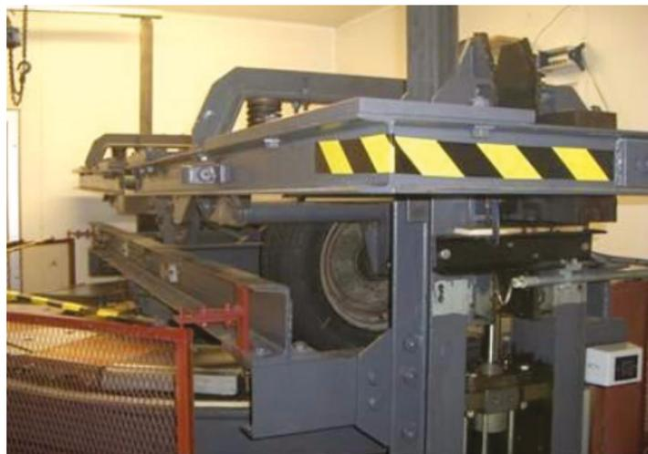
Figure 6 - Road Test machine at University of Ulster
