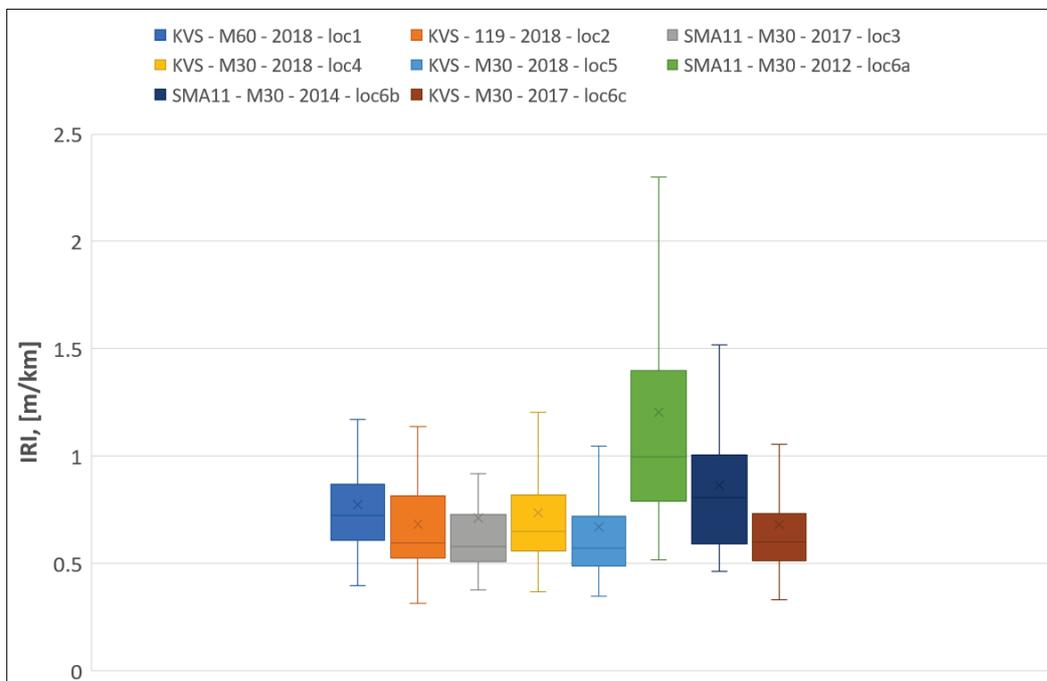
Figure 18 – IRI measured in April 2019 by M+P
