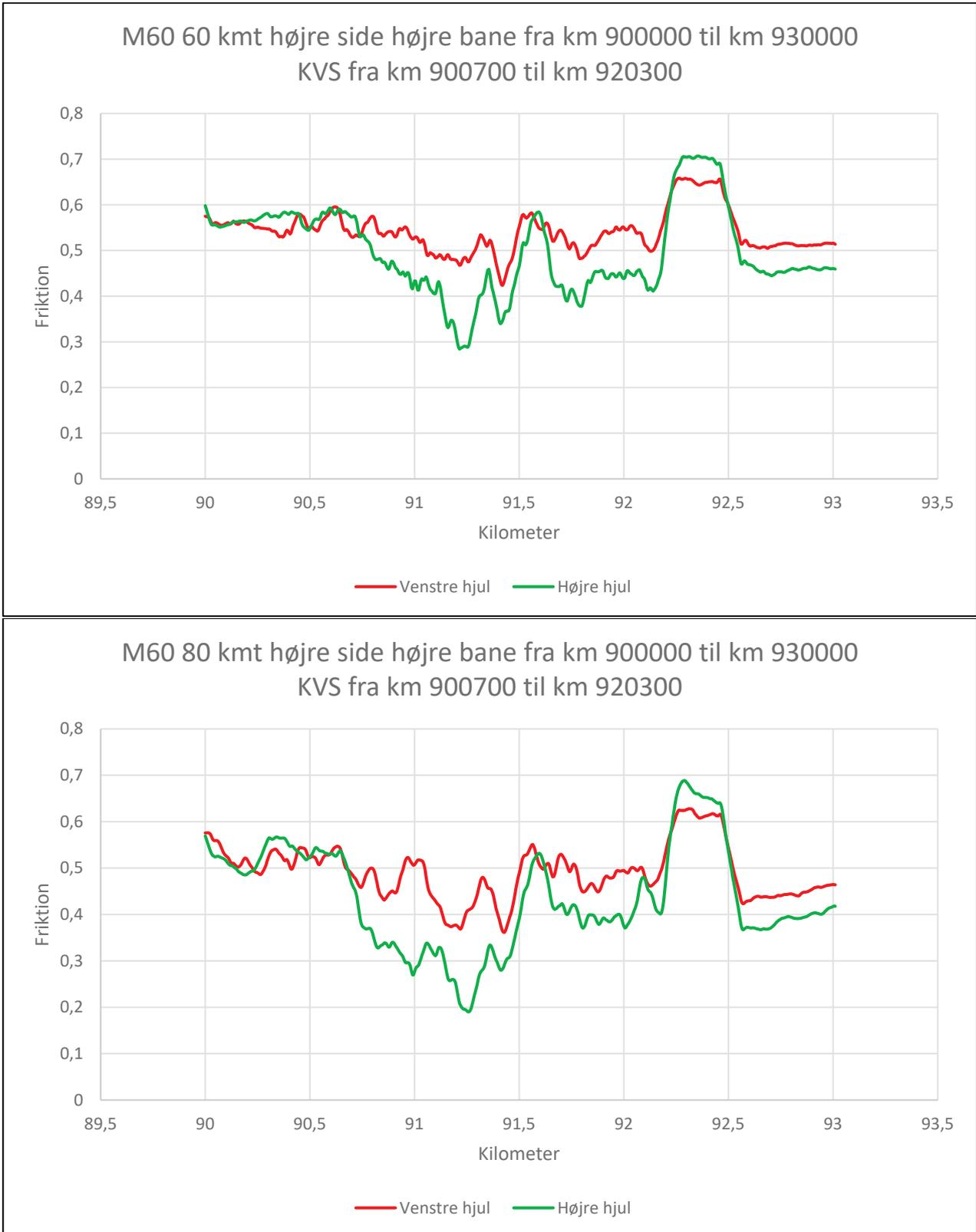
Figure 17 - Friction on M60, right side and right lane at 60 (top) and 80 km/h (bottom).
