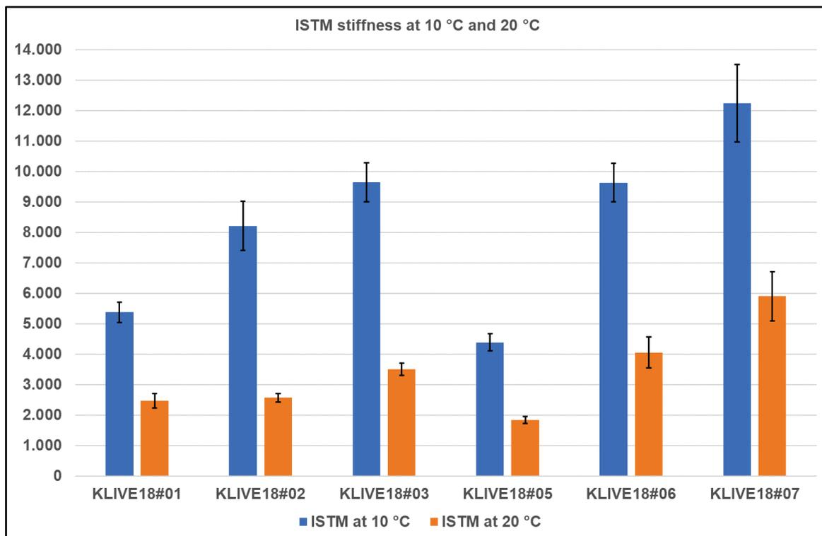
**Figure 4 - Indirect Tensile Stiffness Modulus at 10 °C and 20 °C**
