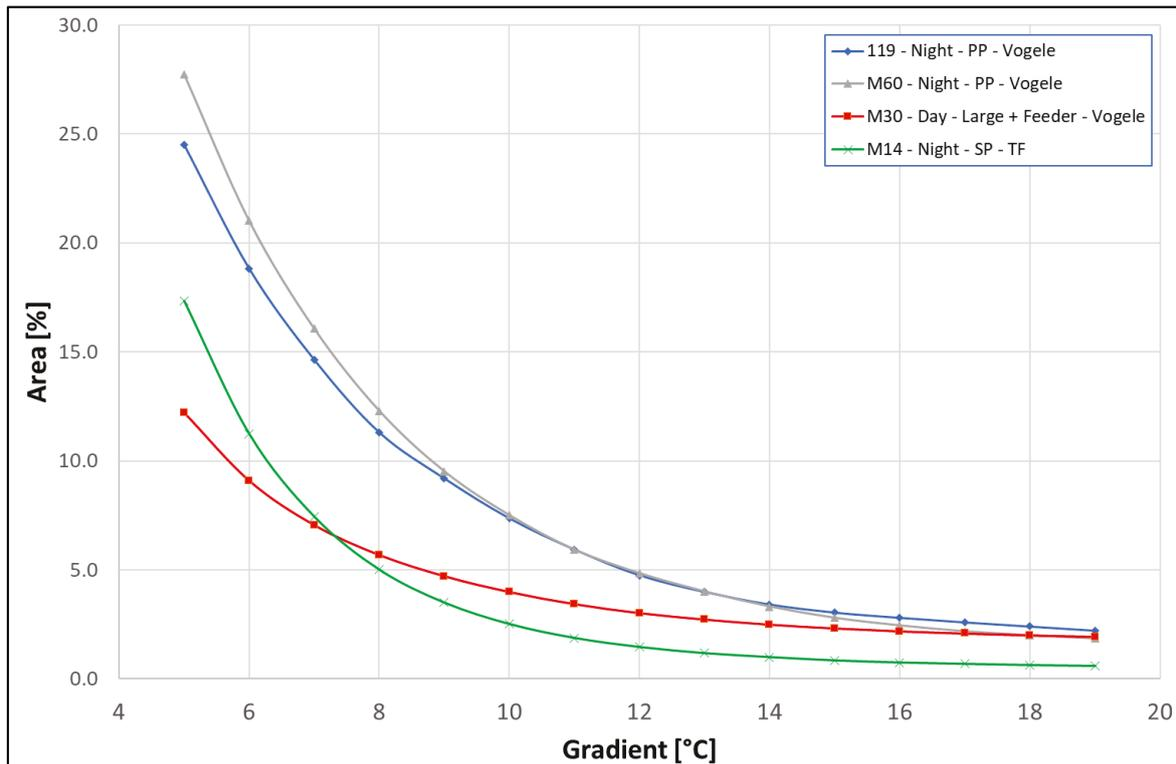
Figure 12 – Temperature gradient and relative percentage of area
