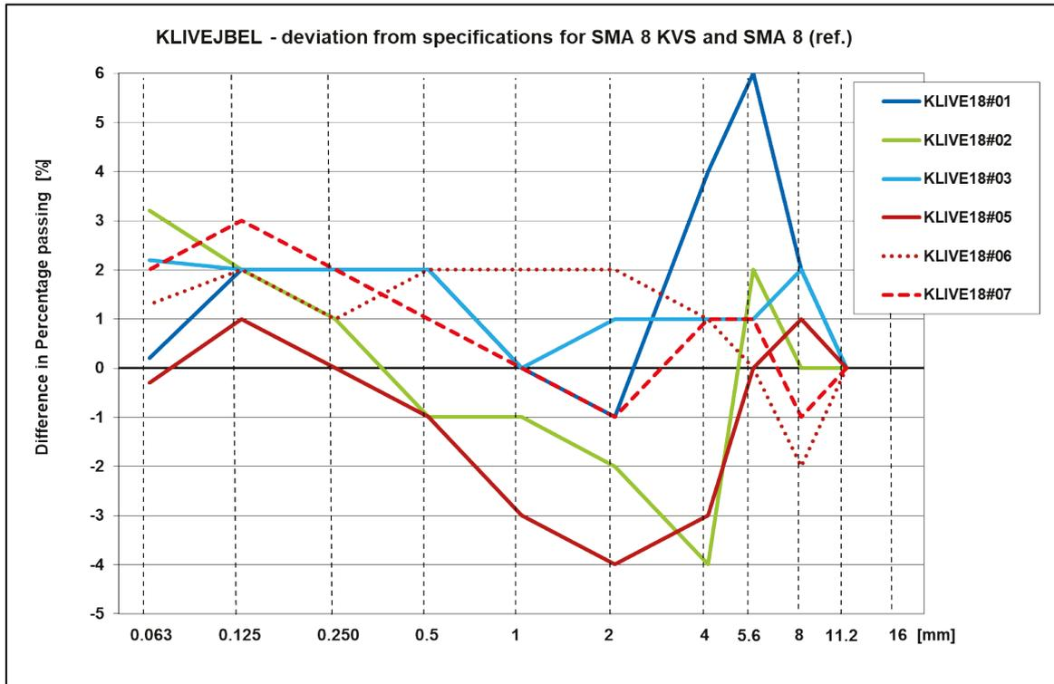
Figure 2 - Difference between the analysed grading curve and the specified grading curve
