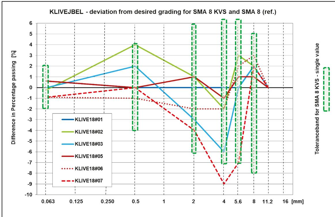
Figure 3 - Deviations from the desired target grading curve of the SMA 8 KVS (see Annex A) and the analysed grading curve including the tolerance bands from DS/EN 13108-21:2016 for single values.
