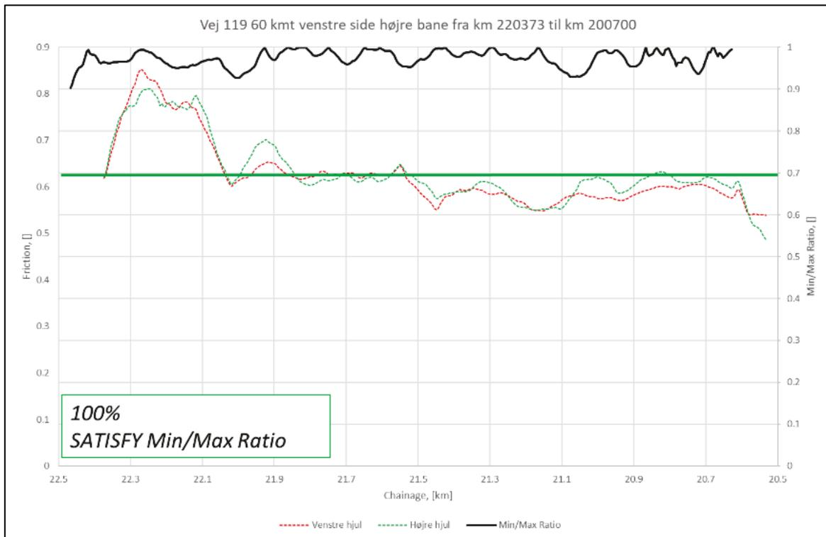
Figure 14 - Surface quality using friction data on Vej 119
