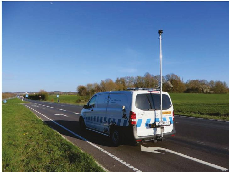
Figure 30 - M+P fc measurement equipment
