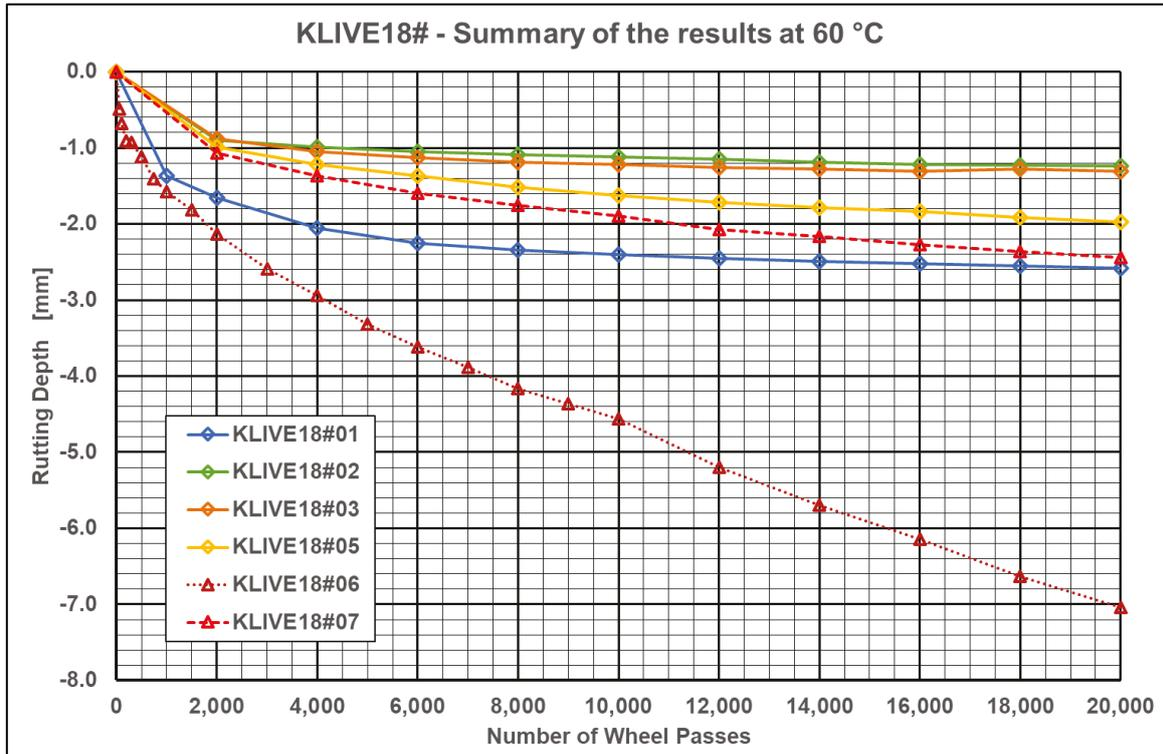
Figure 5 – summary of the results obtained from wheel tracking test at 60°C
