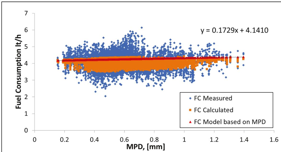
Figure 32 – FC regression model as function of MPD
