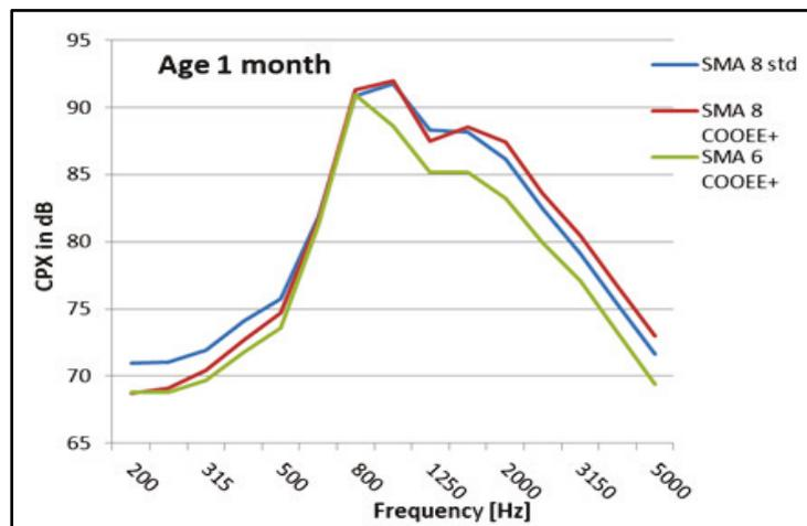
Figure 23 Noise spectra from KVS pavements measured with CPX trailer in 2016 on KVS paved in Kalvehave.
