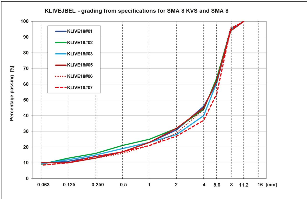
Figure 1 - Grading curves from the asphalt contractors' specifications
