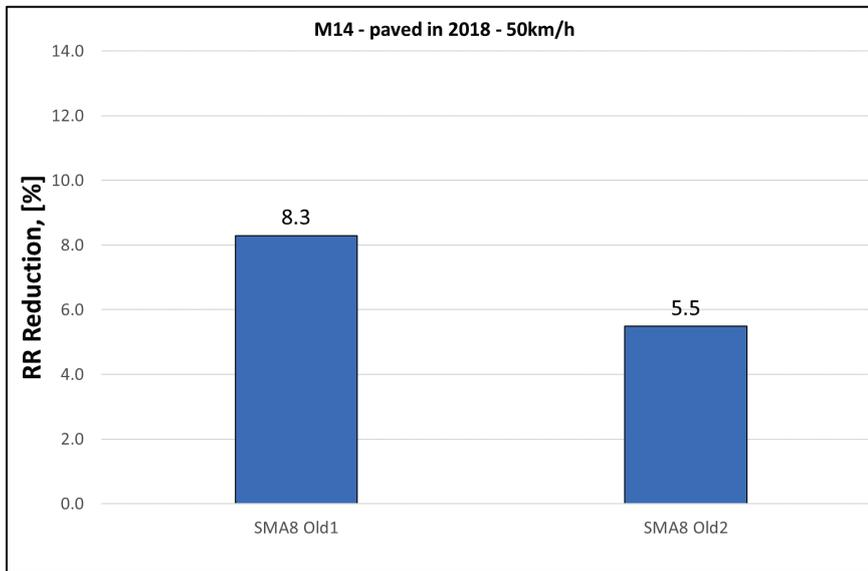
**Figure 29 - RR reduction compared to SMA8 standard – 50km/h**
